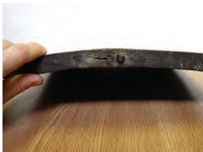
▼ Fig. 3. The curvature of the panel following the loss of the crossbars.
